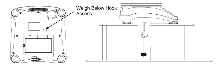
Figure 4-1. Setup for the Weigh Below Hook
