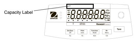
Figure 5-1. Capacity Label location
